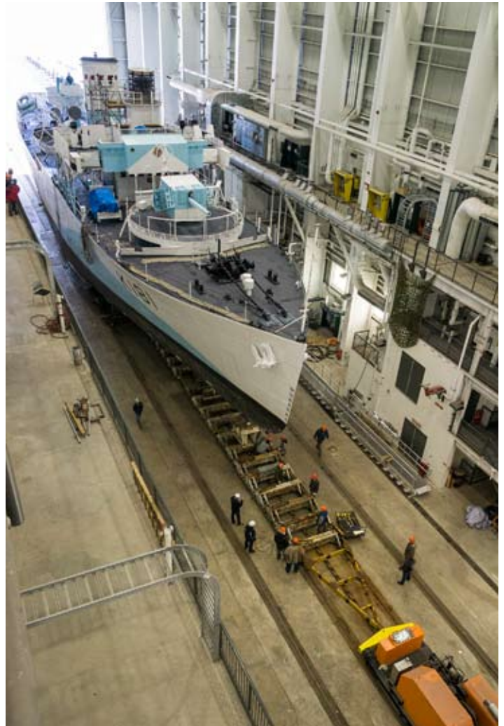
Pulling itself along a heavy chain, the orange tow motor transfers Sackville into the modern Captain Bernard Leitch Johnson submarine maintenance facility.
