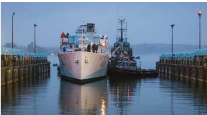
QHM tugs easing Sackville onto Syncrolift.
