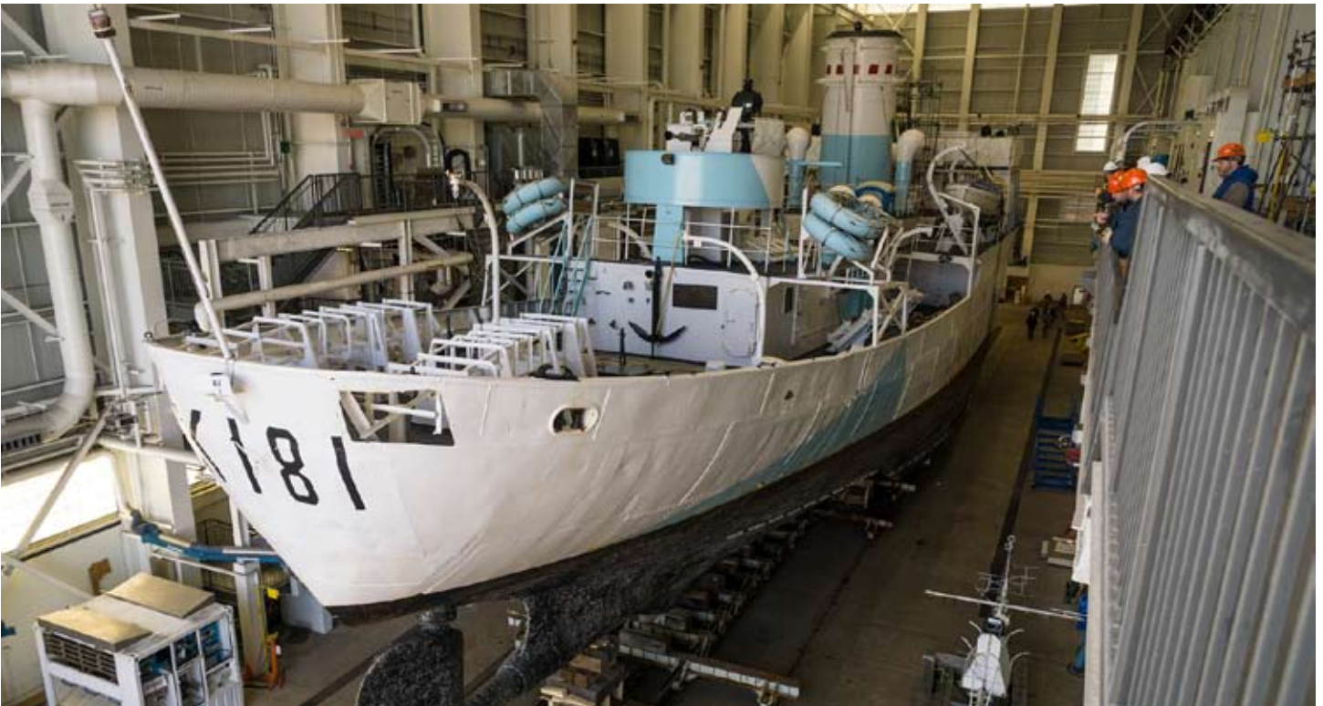
Pulling itself along a heavy chain, the orange tow motor transfers Sackville into the modern Captain Bernard Leitch Johnson submarine maintenance facility.
