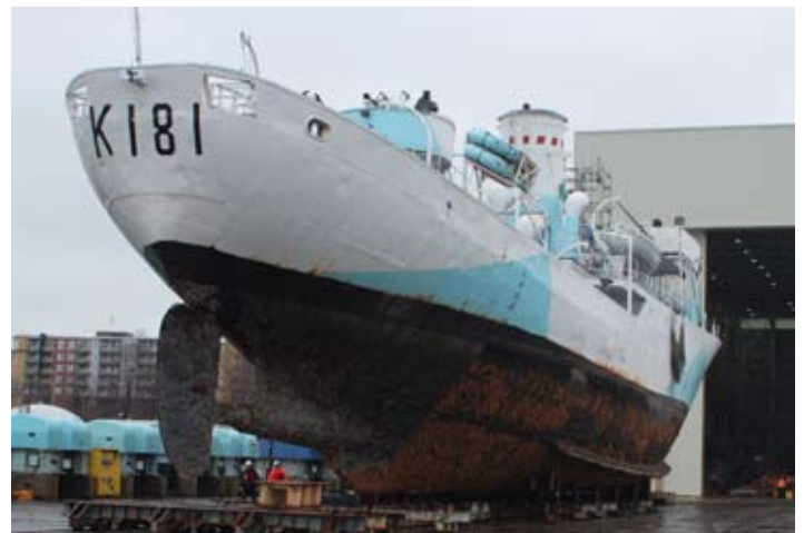
Photo from aft illustrating the level of marine growth in less than a year.
