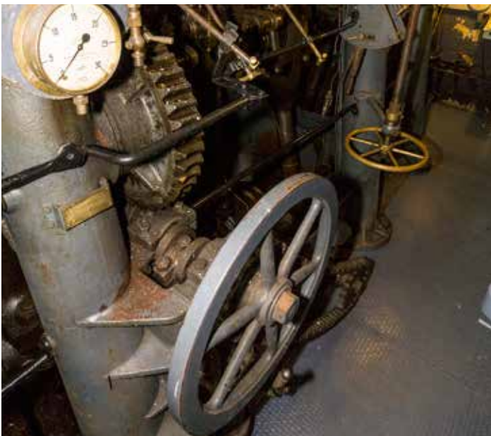
A closeup of the reversing engine, with the throttle handwheel to the right. The throttle handwheel controls a valve at the base of the Aiton bend that regulates the supply of steam to the engine.
