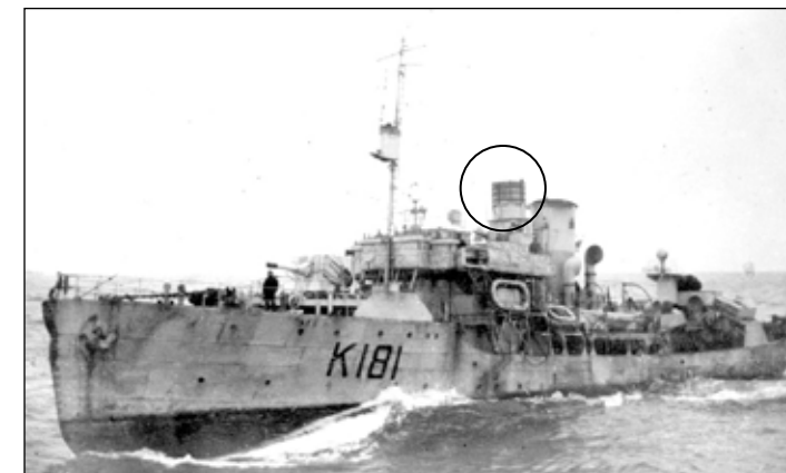
HMCS Sackville's radar housed directly forward and above the funnel.
